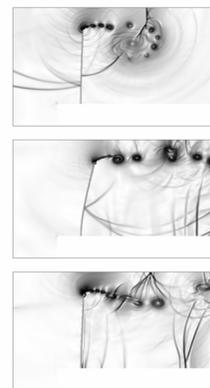
Right: Schlieren plot of fluid density in the vicinity of the thin steel panel. Snapshots for  $t=0.51ms$ ,  $1.63ms$ , and  $3.02ms$  (from top to bottom). Vortex shedding from panel tip and beam vibration induced by shock impact.
