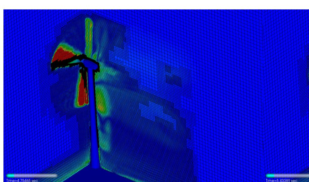
Axial velocity -  $u = 8 \text{ m/s}$ , 33 rpm
