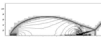
Cartesian base grid 360 × 160 cells on domain of 36 mm × 16 mm with up to 3 refinement levels with  $r_f = 2, 4, 4$  and  $\Delta x_{1,2} = 3.125 \mu m$ , 38 h CPU
