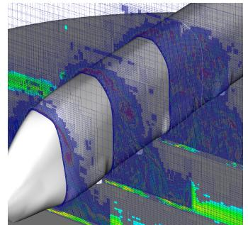
Adaptive LBM code 16x faster than OpenFOAM with PISO algorithm on static mesh!
