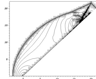
GFM base grid 390 × 330 cells on domain of 26 mm × 22 mm with up to 3 refinement levels with  $r_f = 2, 4, 4$  and  $\Delta x_{e,1,2} = 2.849 \mu m$ , 200 h CPU
