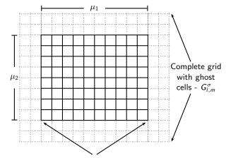
Interior grid with buffer cells -  $G_{l,m}$
