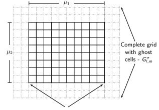
Interior grid with buffer cells -  $G_{l,m}$
