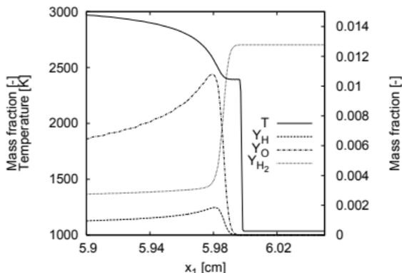
Approximation of  $\text{H}_2 : \text{O}_2$  detonation at  $\sim 1.5 \text{ Pts}/l_{ig}$  (left) and  $\sim 24 \text{ Pts}/l_{ig}$  (right)
