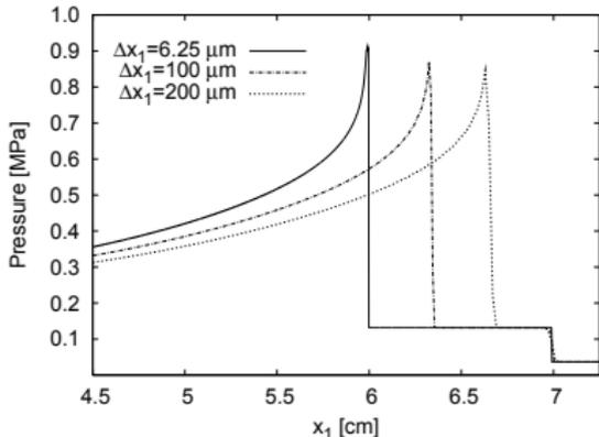
Left: Comparison of pressure distribution  $t = 170 \mu s$  after shock reflection.
